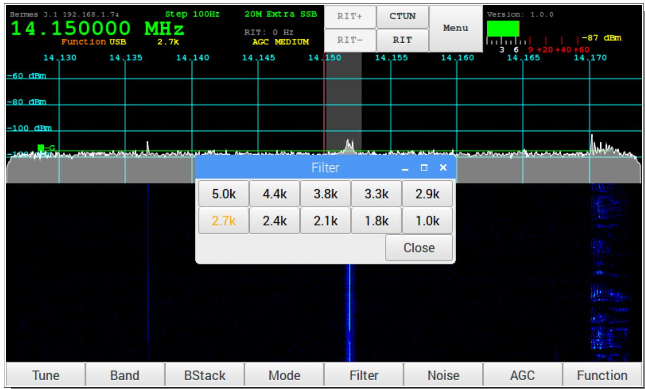
Tapping the Filter touch screen button or pressing the physical button will display the list of filters with the current filter highlighted in orange.
