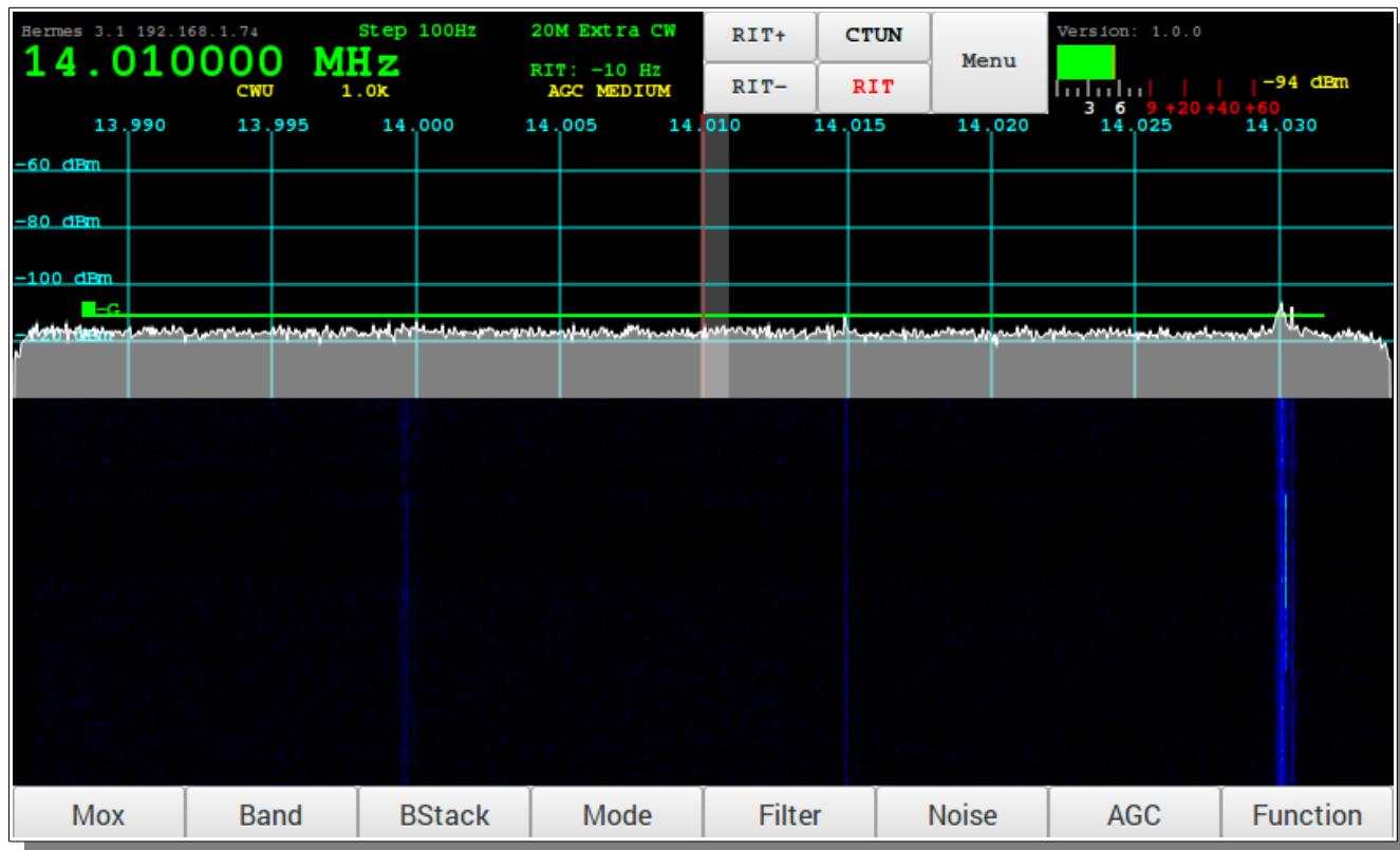
**Tapping on the RIT button will enable RIT.** The RIT+ and RIT- buttons can be tapped or held to increment/decrement the RIT frequency in Hz.
