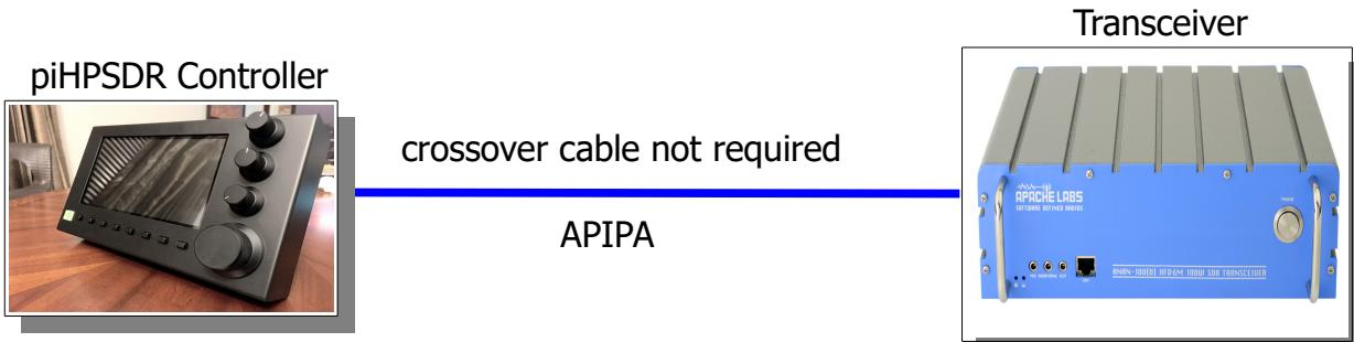
The new piHPSDR-Controller can be connected directly to your ANAN Transceiver and each unit will make use of the APIPA assignment for an IP address.
