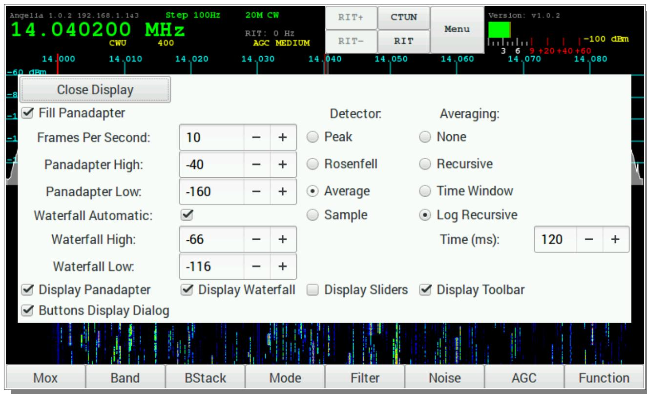
● **Fill Panadapter** – when enabled the panadapter graph will be filled. When not enabled it will be drawn as a line.
