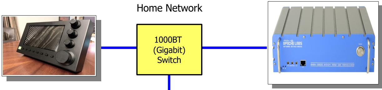
CAT-5 or CAT-6 shielded cables are recommended for connection of the Controller
