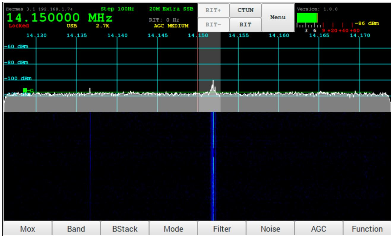
The VFO can be locked by pressing the button on the AF Gain encoder or by tapping on the left side of the VFO display. To unlock press the AF Gain encoder button again or tap on the left side of the VFO display. **When locked the text will be displayed in Red** on the VFO.
