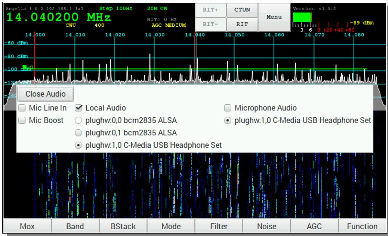
● **Mic Line In** – When enabled the audio from the radio will come from Line In rather than the microphone socket.
