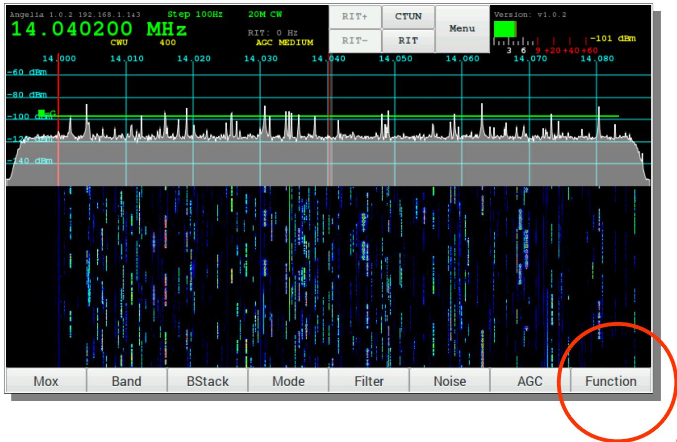
The function touch screen button or physical button enable the optional functions of some of the buttons and encoders.
