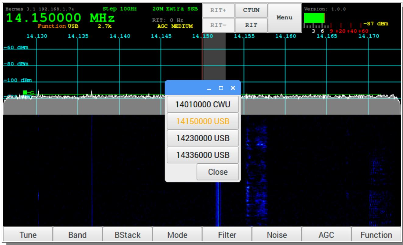
Tapping the BStack touch screen button or the physical button will display the list of Band Stack entries for the current band with the current selection highlighted in orange.
