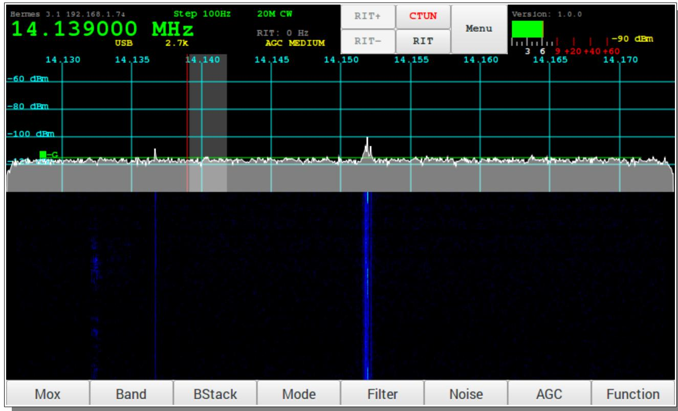
Tapping on the CTUN button will enable or disable the click tuning function. When the function is enabled the CTUN button text will be red.
