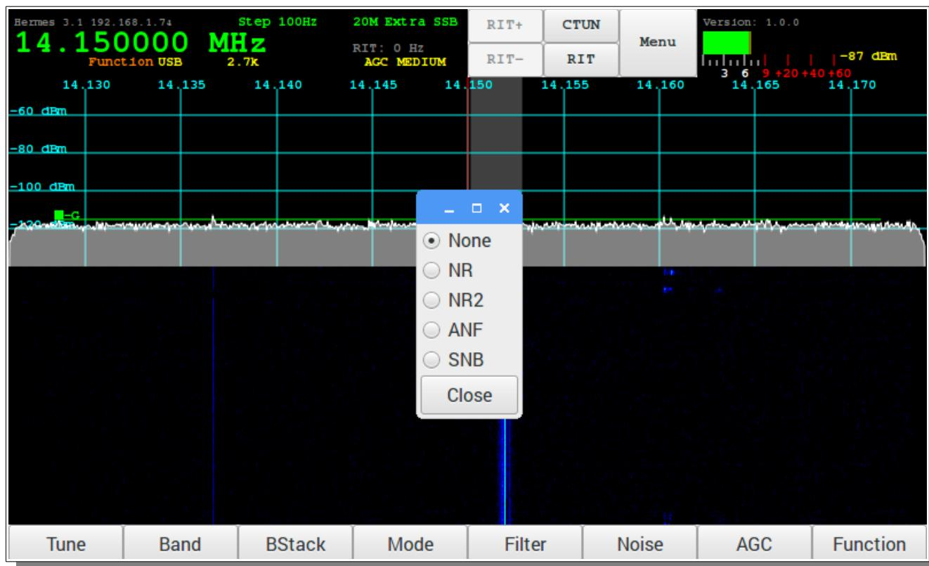
Tapping the Noise touch screen button or physical button will display the list of noise reduction modes are available.
