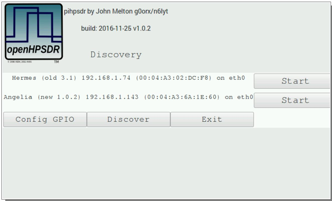
If no devices are found you should check connectivity between the radio and the network that piHPSDR is connected to. Tapping on OK will try discovery again. Tapping on Cancel will exit piHPSDR back to the Raspberry Pi desktop.
