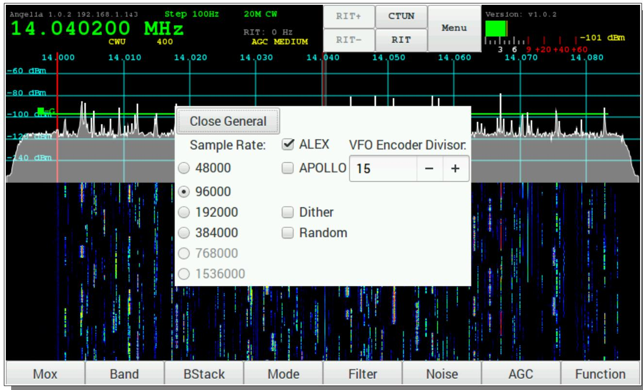
● **Sample Rate** - The Sample Rate selection selects the width of the Panadapter displayed on the piHPSDR Controller screen. This is the rate which **pihpsdr** uses to decode a portion of the 30Mhz spectrum data from the Apache Transceiver.
