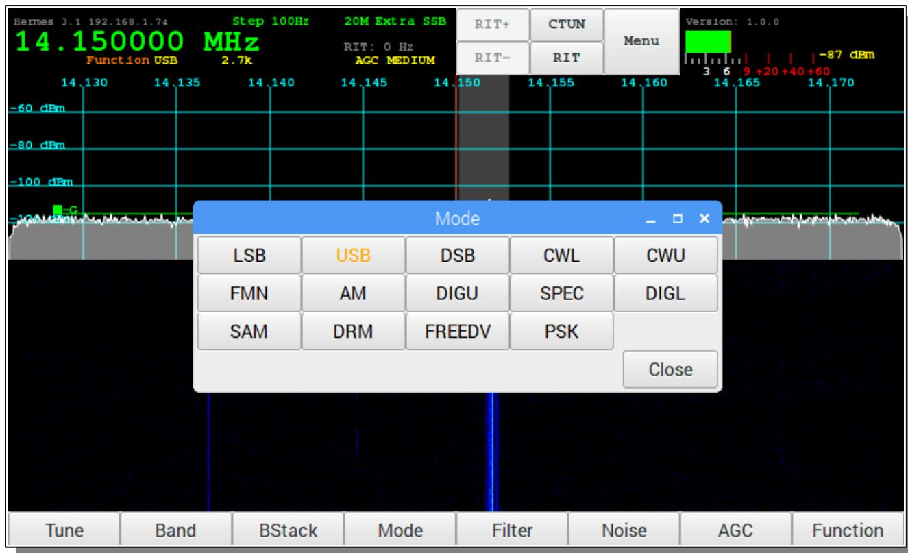
Tapping the Mode touch screen button or pressing the physical button will display the list of modes with the current mode highlighted in orange.
