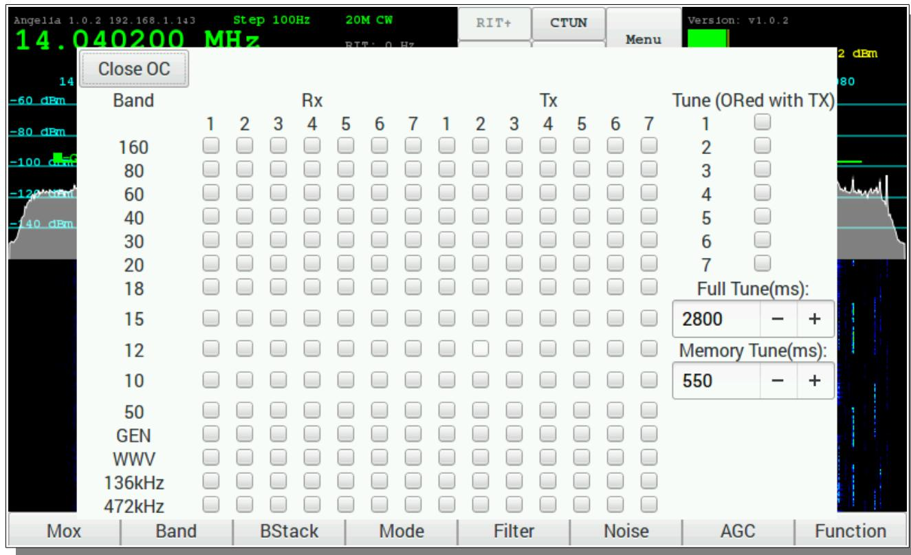
Configure the Open Collector outputs for each band. These can be used to control an external filter when not using the Apache Labs filters or the Alex filters. The default is none are enabled.
