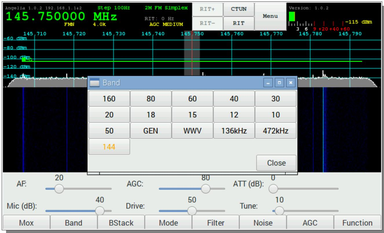
Tapping the Band touch screen button or pressing the physical button will display the list of bands with the current band highlighted in orange.
