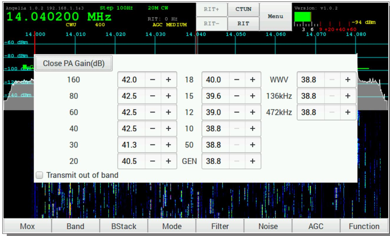
Sets the gain for each band to set the maximum drive level. Note that as the setting are increased the drive level is decreased.
