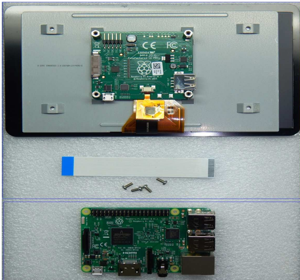
Contents of the Rpi and the official Rpi 7 inch screen kit
